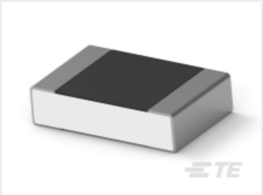
TE Part #5-2176381-8 RQ 0805 48K7 0.1% 10PPM 5K RL
