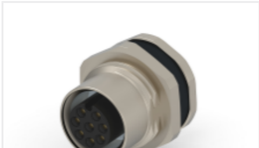
TE Part #T4171120008-001 M12,REAR MOUNT,FEMALE,A,8P,0.2 M WIRE
