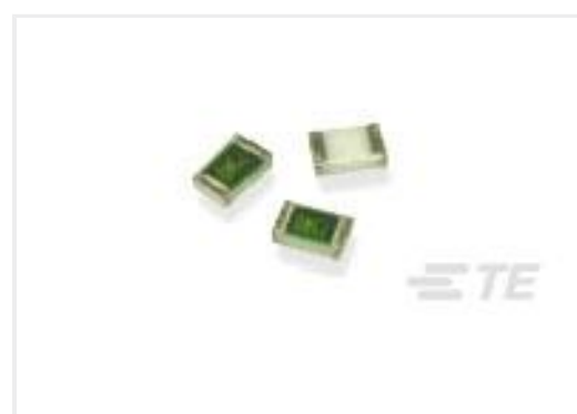
TE Part #1676220-1 RN 0805 1K07 0.1% 10PPM CUT LE
