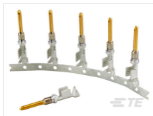
TE Part #2098252-1 PIN, SF, SIZE 16, 14-16 AWG, AU/SN
