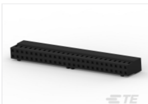
TE Part #5-2316109-0 50P, 2MM, REC, HSG, DR, CRIMP, LCK RAMP, BOX
